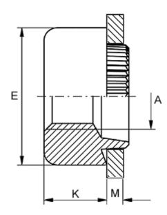
Female thread A = M6Height K = 6.0Outer diameter E = 13.0Plate thickness = 1.7 to 1.9
